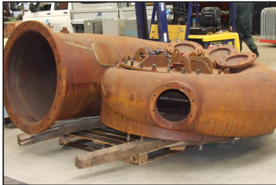
Cast Steel pump built in 1949! With a diameter of 2,5 meter, 30 m 3 /minute
