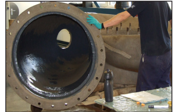
Multiple ARC products used to address various wear levels and surface enhancement
